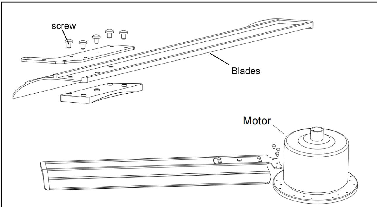
4.1 Tightening the screw with the motor.
