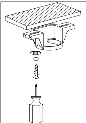
The hanger bracket should be screwed on to a firm flat surface. The fixing location must be able to withstand ten times the static weight of the fan. In most situation two wood screws screwed into a wooden joist is more than adequate to support your ceiling fan
