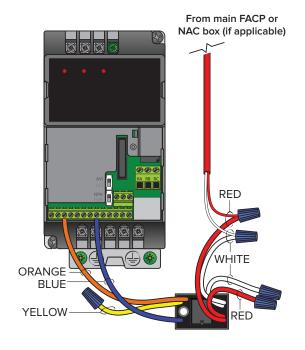
A contact closure across digital input terminals MI3 and DCM will result in fan shutdown. The relay uses a Normally Open (N.O.) contact. The relay coil must be energized by the FACP for fan shutdown.
