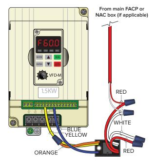
Optionally, the relay can be used with a Normally Closed (N.C.) contact. The relay coil must remain energized by the FACP for fan operation. This would be considered a fail safe or fail open wiring arrangement.
