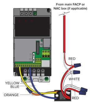
Optionally, the relay can be used with a Normally Closed (N.C.) contact. The relay coil must remain energized by the FACP for fan operation. This would be considered a fail safe or fail open wiring arrangement.
