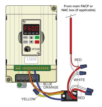
A contact closure across digital input terminals M3 and GND will result in fan shutdown. The relay uses a Normally Open (N.O.) contact. The relay coil must be energized by the FACP for fan shutdown.
