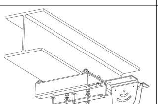
Secure the yoke to the I-beam with 4 sets of yoke M10x50L 4 bolt kit.
