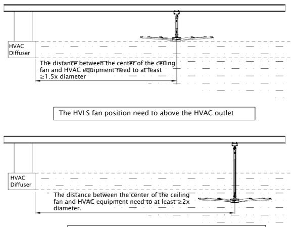
The HVLS fan position need to below the HVAC outlet
